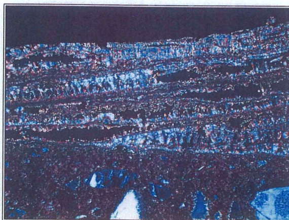
Sample S2: Laminated \text{CaCO}_3 crystals on the surface of the concrete. The width of the field is 3.88mm under crossed polarised light.
