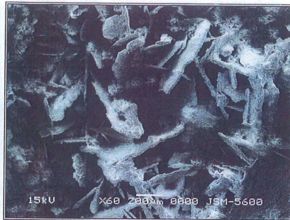
Sample S3: Secondary electron image (SEI) showed coarse-grained flaky crystals in the crack.
