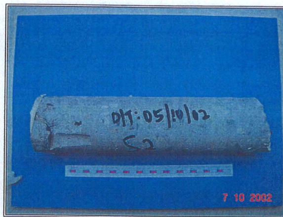
Relative thick whitish substance was on the surface of core S2.
