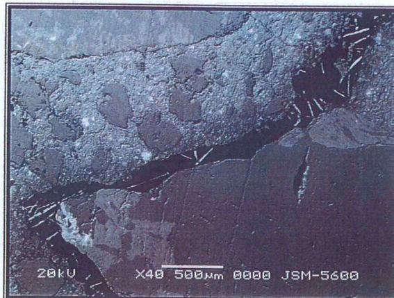
Sample S3: Backscattered electron image (BEI) showed some crystals was in the crack.
