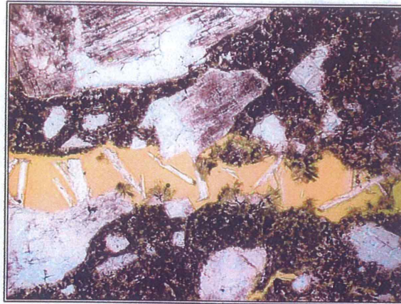
Sample S3: Coarse-grained elongated crystals and fine-grained needle-like crystals were lining the crack. The width of the field is 3.88mm under plane light.
