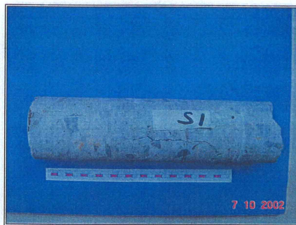
A crack perpendicular to the exposed surface was seen in core S1.
